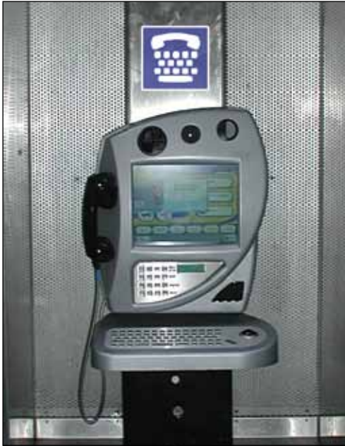
Image 6.7 Example of a textphone located at a public payphone.
