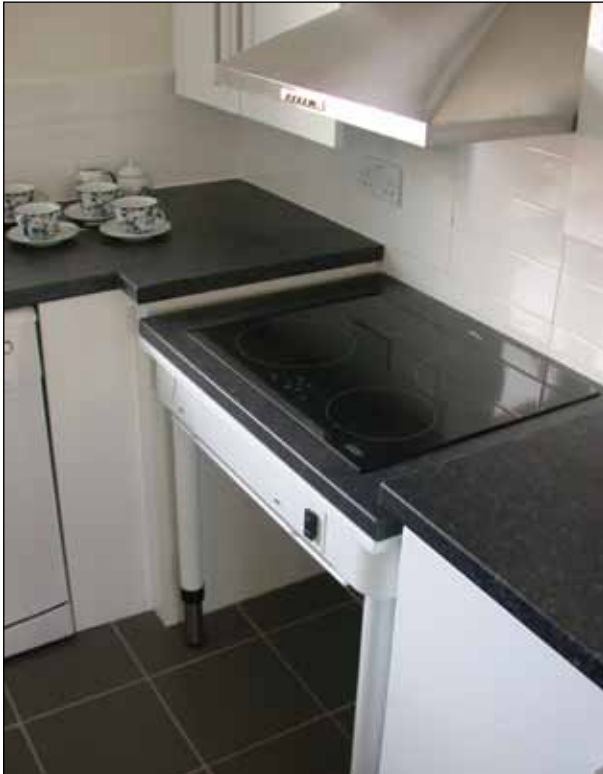
Image 6.13 Example of an accessible ceramic hob.
