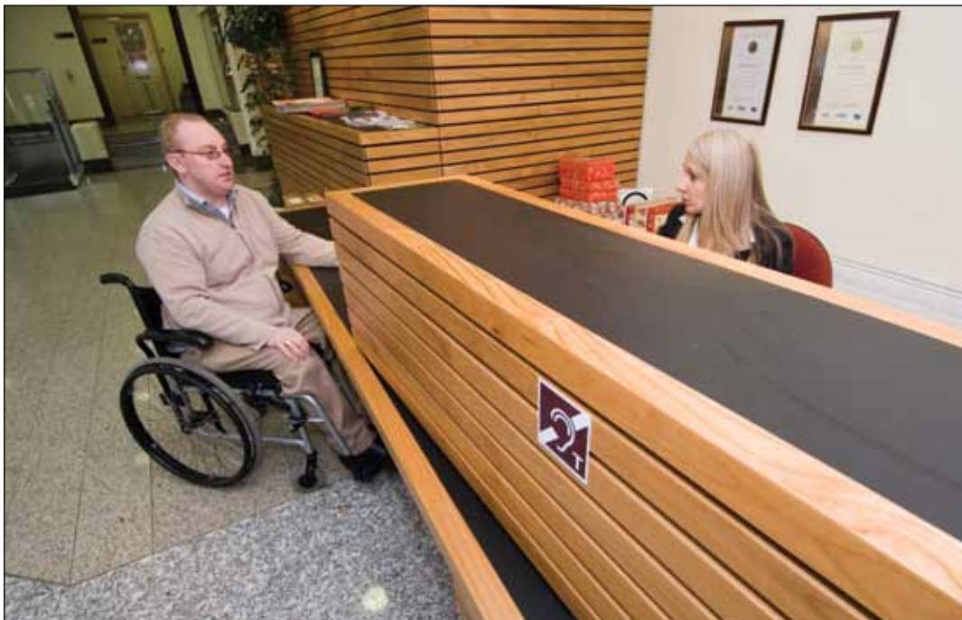
Image 6.3 Alternative view of a reception desk with two levels.
