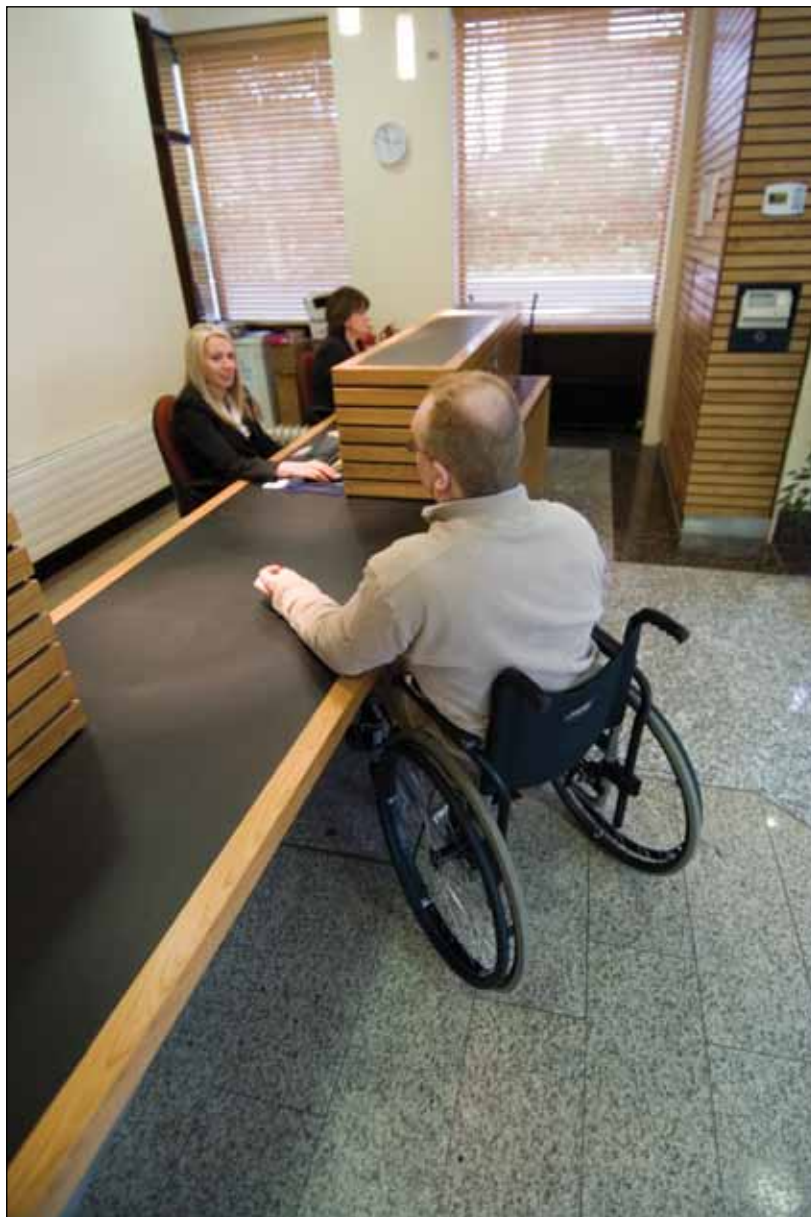
Image 6.2 Example of a reception desk with two levels.
